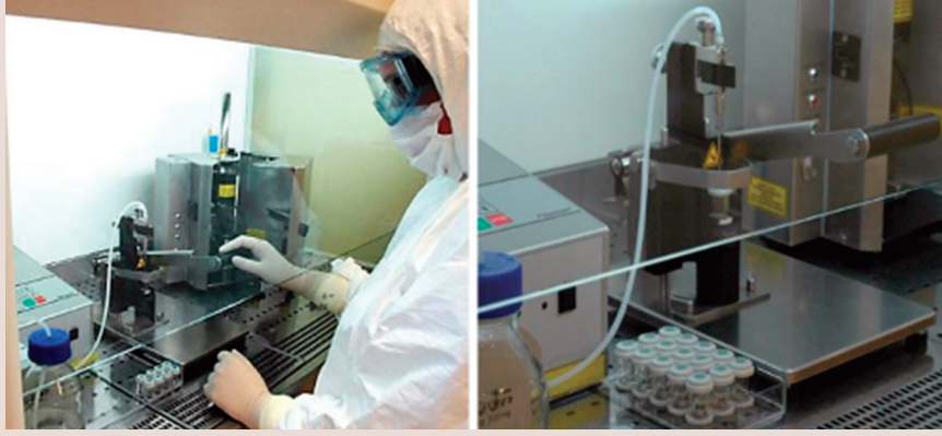
Figure 4: (LEFT) the M1 filling system; (RIGHT) a close-up view of the dispensing needle
